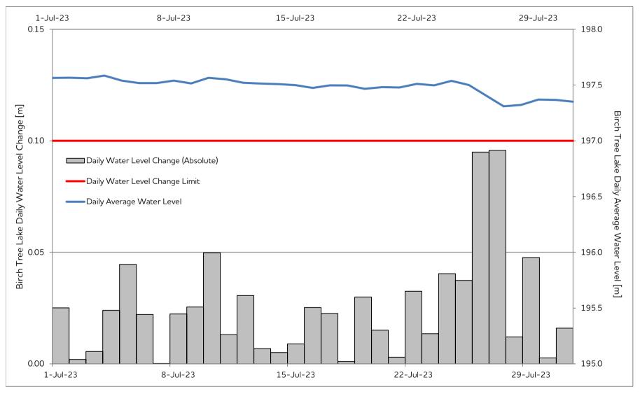
Note: The Birch Tree Lake Daily Water Level Change is calculated using Birch Tree Lake gauges 05TG701, 05TG746 The daily water level change limit is equal to 0.1 m in open water conditions (May 1 to October 31) and 0.15 m in winter conditions (November 1 to April 30)
